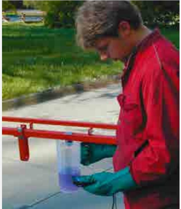
Even with flow-controlled devices, a water capacity test is necessary. Source: Bildungswerkstatt Mold, Pichler Herbert
