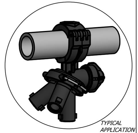
TO INSTALL NOZZLE BODY, DRILL 3/8" (9.5MM) DIA. HOLE IN PIPE, DEBURR, THEN INSERT SPLIT-EYELET INLET AND CLAMP ASSEMBLY IN PLACE
